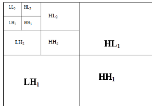
Fig.1 Three phase decomposition using DWT
